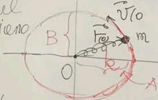
$$\vec{F} = -k\vec{r} \quad \left\{ \begin{array}{l} m\ddot{x} = -kx \\ m\ddot{y} = -ky \end{array} \right. \quad \omega_0 = \sqrt{\frac{k}{m}}$$
